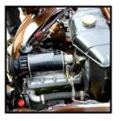
The Topolino was equipped with a small 560 cc four-cylinder, water-cooled engine -- which sounded like a high-class sewing machine ... Nevertheless, it was a full-scale car, and quite funny to drive!
